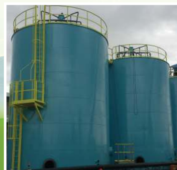
Biogas Upgrading and H 2 S Bio-Scrubber System, Ethanol Factory
