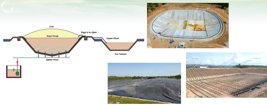
MCL technology is developed from conventional anaerobic lagoon that can overcome problems of sludge sediment at lagoon problem. The process starts by entering wastewater from the bottom level of MCL to mix with microorganism (anaerobic sludge). The substrates inside digester will be automatically circulated through networks of solenoid actuator valves and piping, and sediment sludge will be collected at the end of the lagoon.
