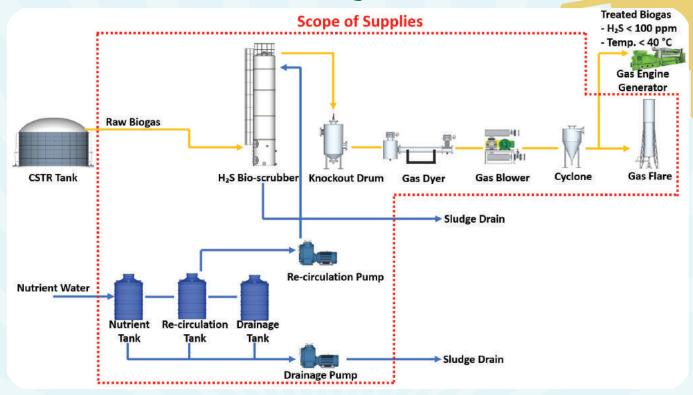
Biogas is normally comprised of mixed types of gases, i.e. Methane ( $CH_4$ ), Carbon Dioxide ( $CO_2$ ) and Hydrogen Sulfide ( $H_2S$ ) gases. The content of  $H_2S$  in raw biogas is typically in the range of 1,000 – 20,000 ppm, which its combustion and humidity in gases can produce Sulfuric Acid and leads to severe corrosion of engine parts, valves and pipes in biogas systems.
